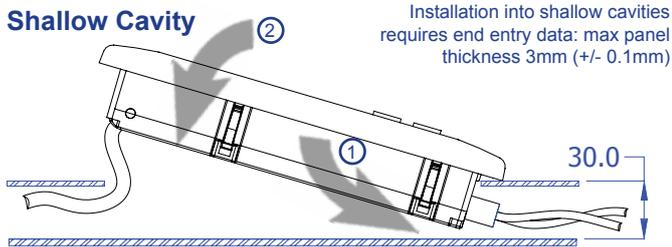
Data is hardwired from PUMA in thin cavity situations
